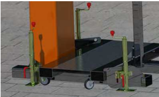
Casters and adjustable legs permit easy positioning
